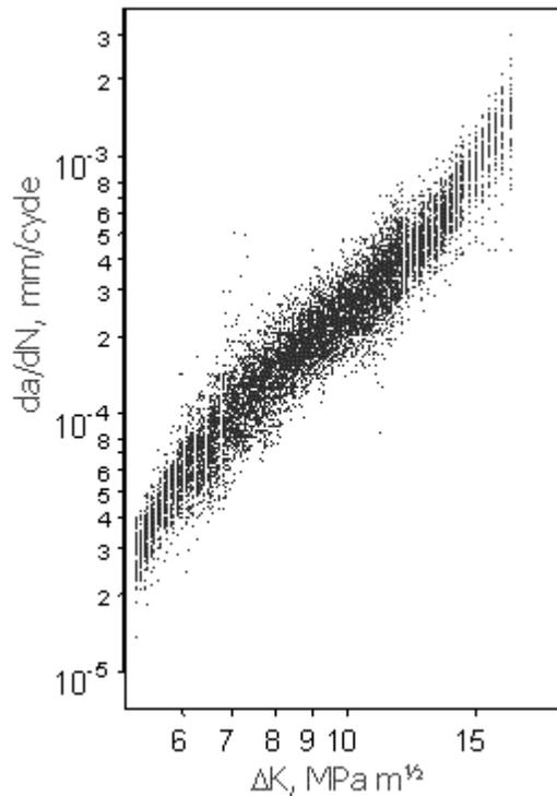
Figure 1 -  $da/dN$  vs.  $DK$  are S-shaped.
