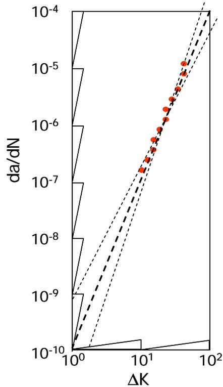
Figure 3 - Schematic showing why Paris Parameters must be correlated. Note that in this schematic the intercept is  $C = \log_{10}(da/dN) = -10$ , at  $\log_{10}(DK) = 0$ .
